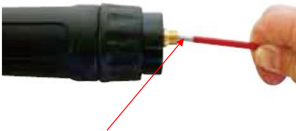
(5) Carefully feed in the new liner down the torch lead all the way to exit the torch neck.
