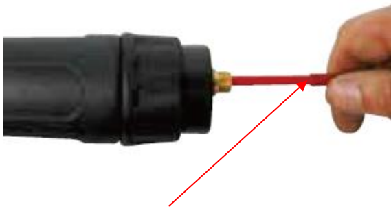
(3) Carefully pull out and completely remove the liner.
