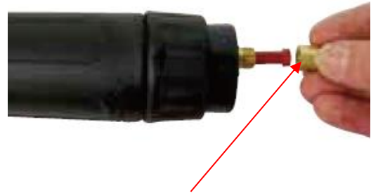
(2) Remove the liner retaining nut.
