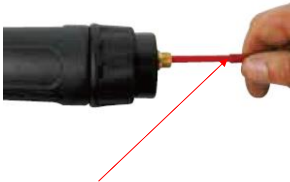
(3) Carefully pull out and completely remove the liner.
