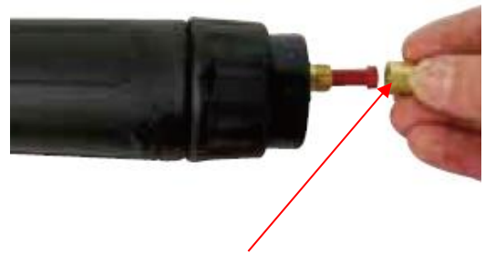
(2) Remove the liner retaining nut.
